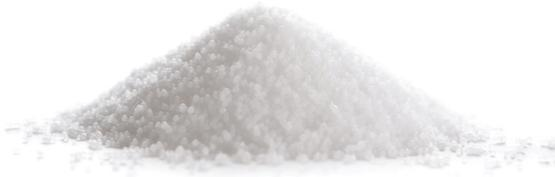
CellBlockEX is 100% recycled material and is made from post-consumer-recycled glass that's destined for the land-fill prior to being diverted to one of two manufacturing plants worldwide.
